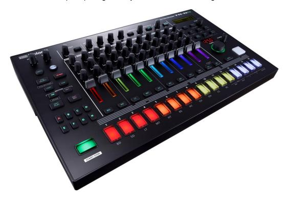
The TR-8S includes many percussion-tuned effects for enhancing individual sounds or entire kits with character, depth, and space. Version 2.0 adds Saturator, Freq Shift, Ring Mod, and Spread effects to the mix, which can be assigned to control knobs for shaping sounds on the fly.
